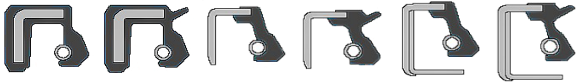
Bauform A Bauform AS Bauform B Bauform BS Bauform C Bauform CS
