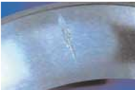
Spalling in the middle of the rolling element path
