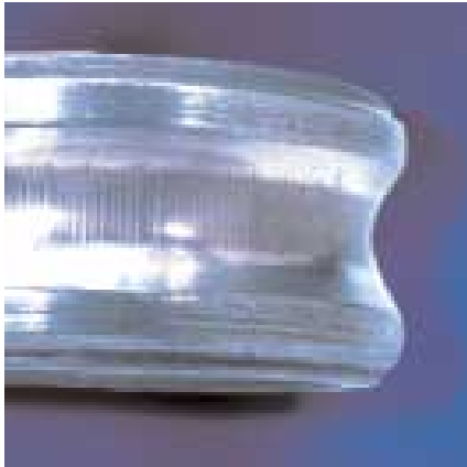
Electric current through the rotating inner ring
