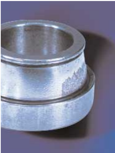
Cone spalling due to misalignment
