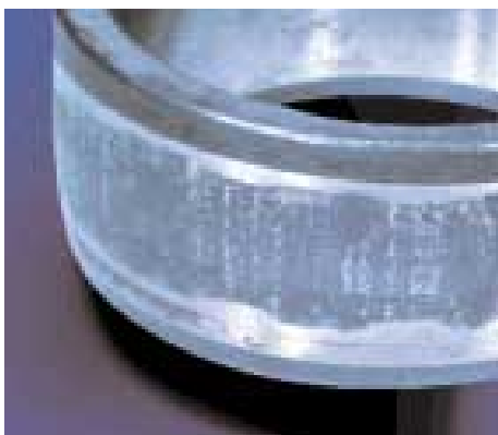
Corrosion when operating (liquid ingress)
