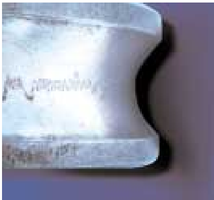
Electric arcing on the inner ring
