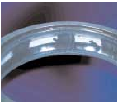
Corrosion when non-operating (liquid ingress)
