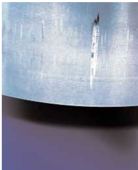
False brinelling on a roller bearing
