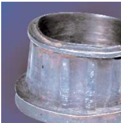
Seizing of a tapered roller bearing with roller imbedding
